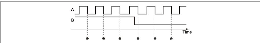
Figure 210: NC150 1 channel, negative edge
