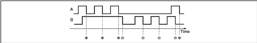
Figure 208: NC150 2 channel, negative edge
