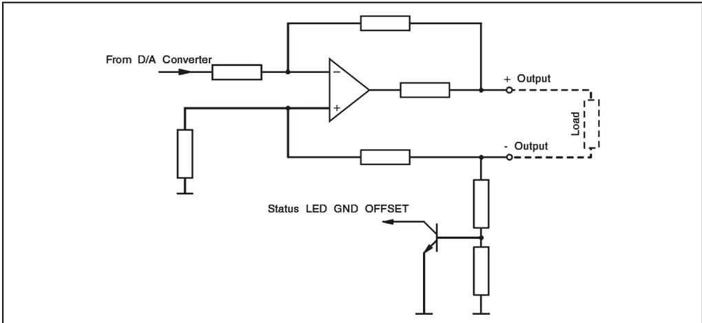
Figure 200: NC150 output diagram for analog outputs
