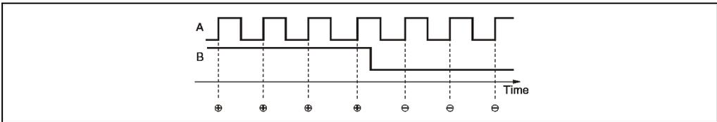
Figure 209: NC150 1 channel, positive edge
