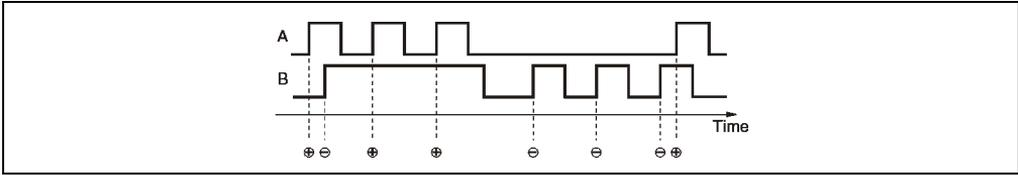
Figure 207: NC150 2 channel, positive edge
