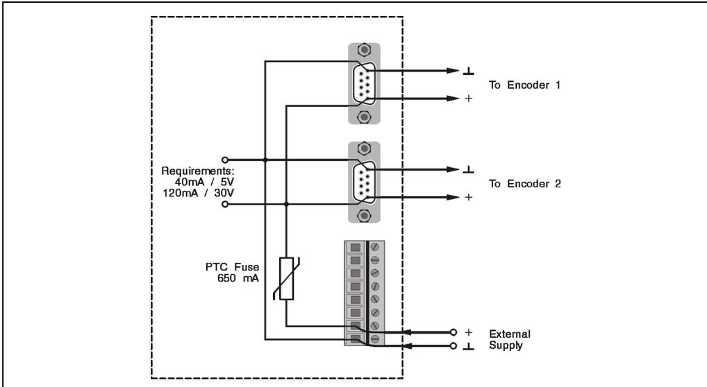
Figure 198: NC150 encoder supply
