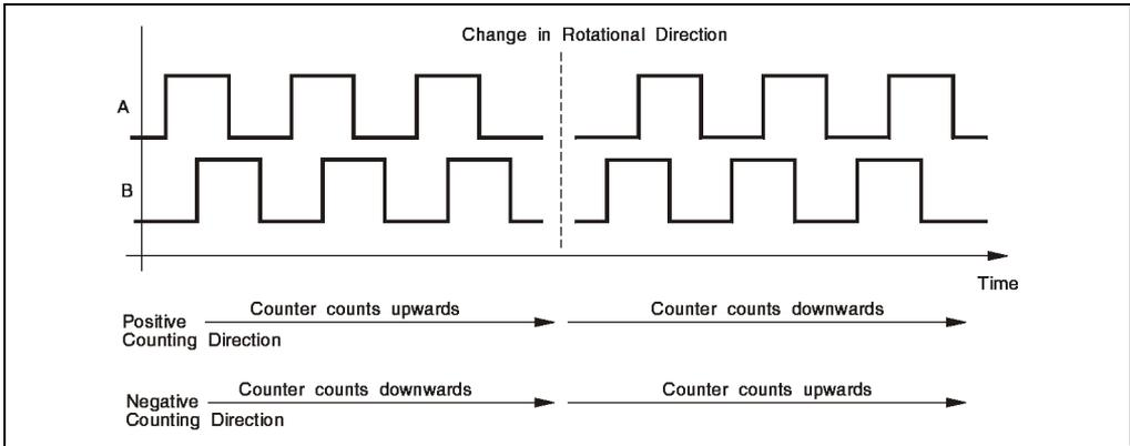
Figure 202: NC150 counting direction in operation mode positioning
