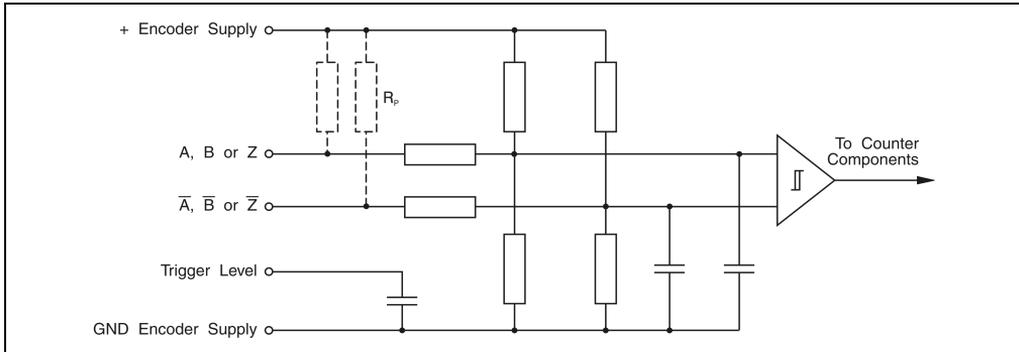
Figure 201: NC150 input circuit for counter inputs
