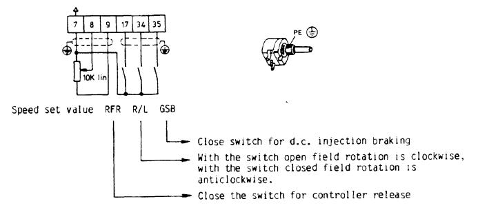
Control inputs are not isolated. Use highly isolated potentiometers. Use 250 V~rated cables.
