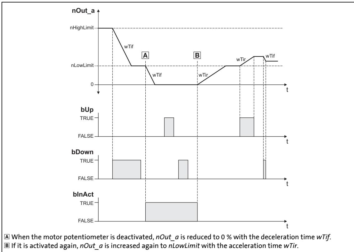
[11-2] Example: Deactivation of the motor potentiometer if [C804](#) = "1: Deceleration to 0"
