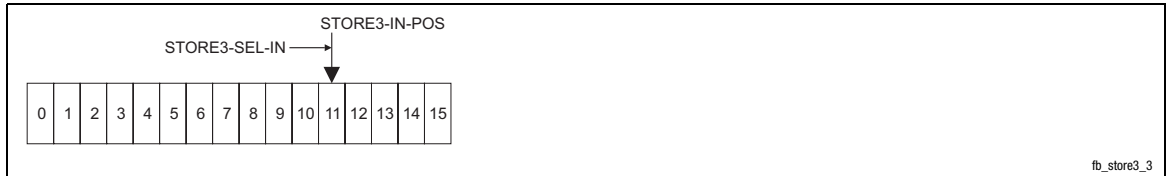
Fig. 3-246 Writing data to a memory location
