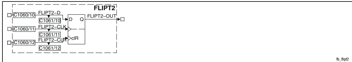
Fig. 3-145 Flipflop element (FLIPT2)
