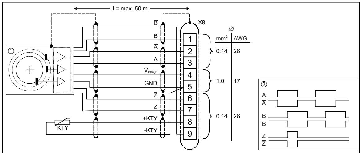
Fig. 4-10 Connection of the incremental encoder to input X8
