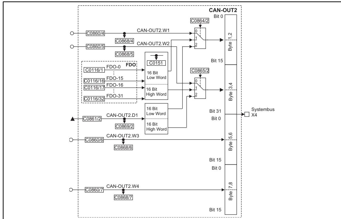
Fig. 7-49 System bus (CAN-OUT2)
