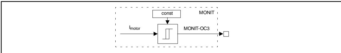
Fig. 7-169 Overload during acceleration or deceleration OC3
