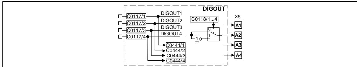
Fig. 7-91 Digital outputs (DIGOUT)
