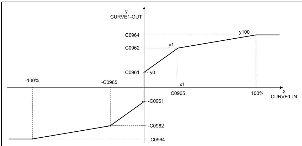
Fig. 7-66 Characteristic with three co-ordinates
