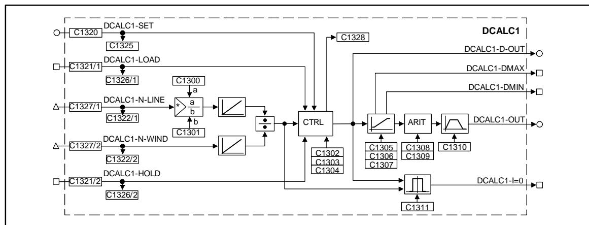
Fig. 7-70 Diameter calculator (DCALC1)
