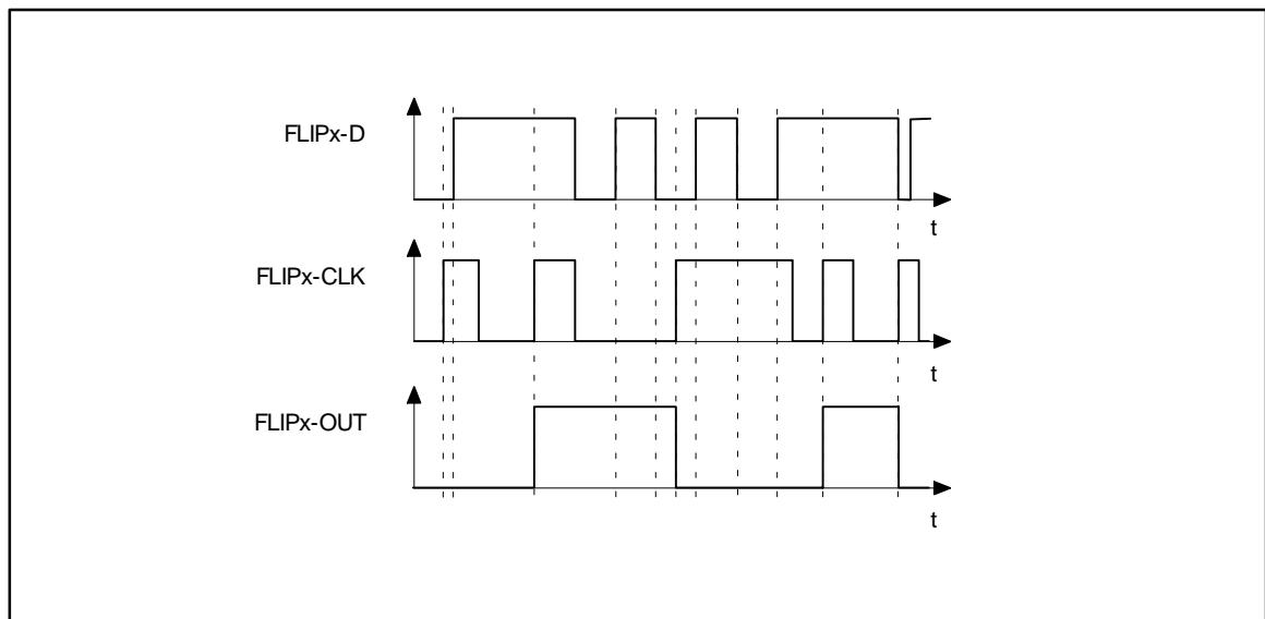
Fig. 7-102 Sequence of a flipflop
