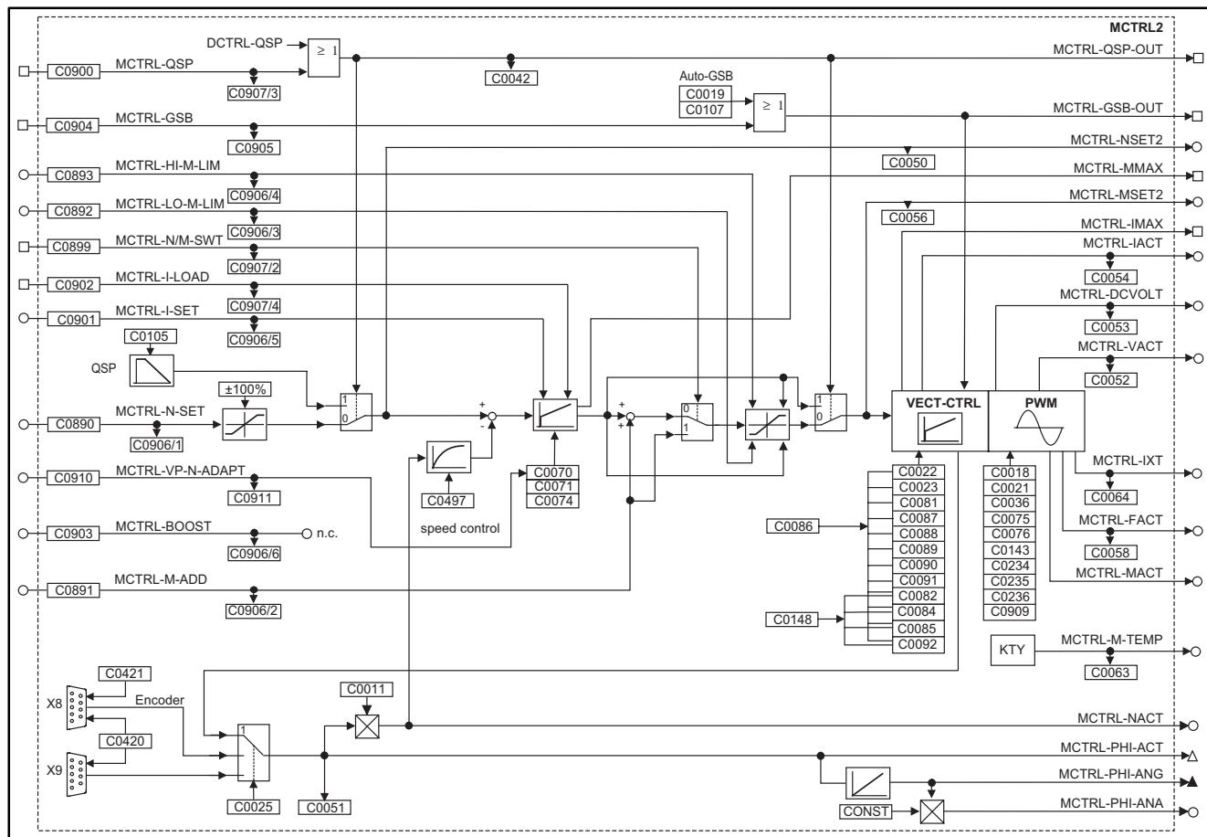
Fig. 7-108 Internal motor control with vector control (MCTRL2)
