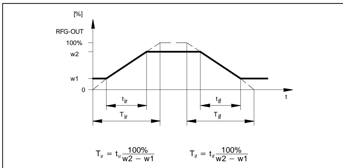
Fig. 7-128 Acceleration and deceleration times of the ramp generator
