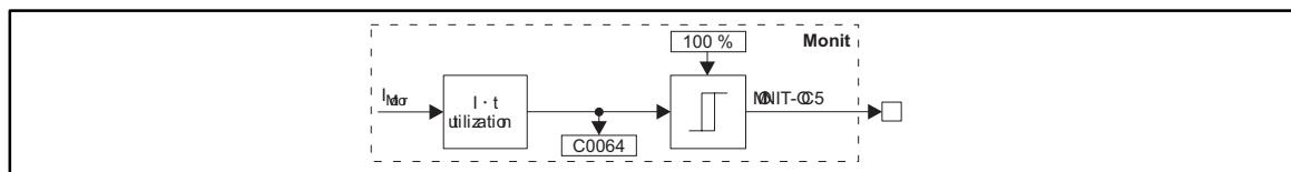
Fig. 7-170 Monitoring of the  $I \times t$  overload (OC5)
