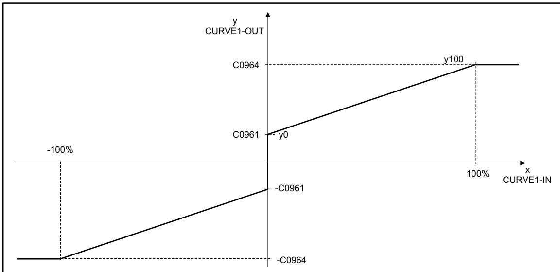
Fig. 7-65 Characteristic with two co-ordinates
