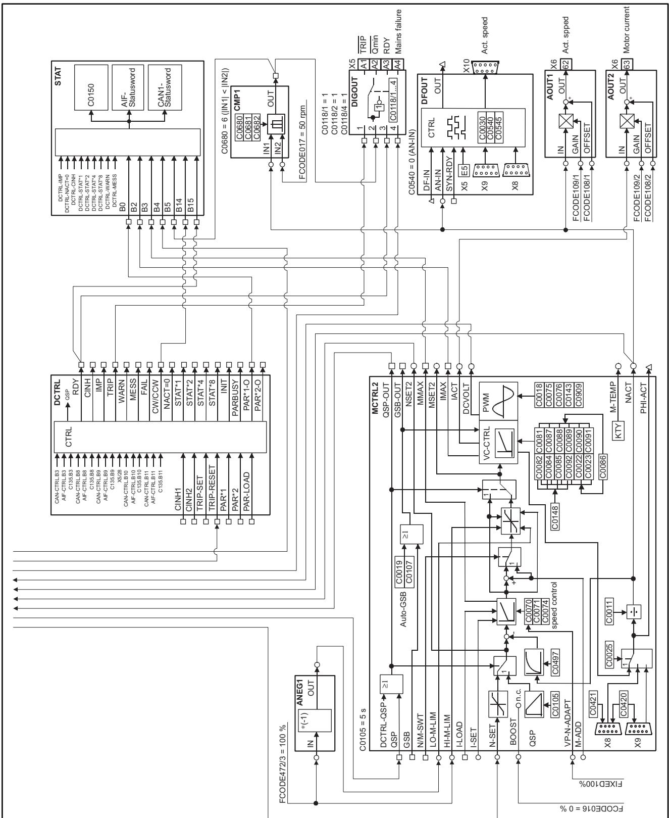
Fig. 16-10 Basic configuration 1400 - speed control with mains failure control (sheet 2)
