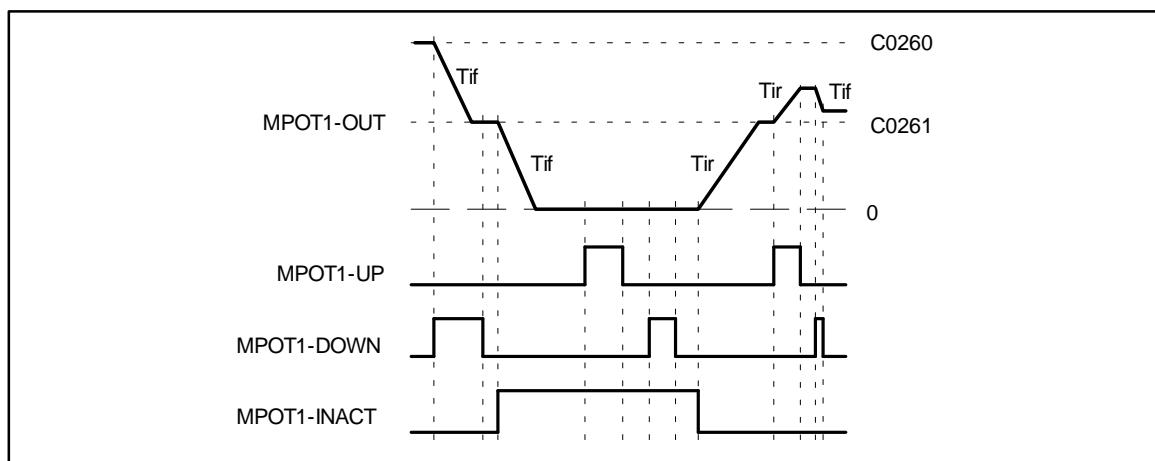
Fig. 7-118 Deactivation of the motor potentiometer via the input MPOT1-INACT
