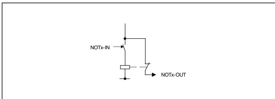
Fig. 7-126 Function of NOT as a change from a normally-open to a normally-closed contact
