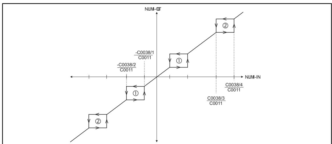
Fig. 7-120 Representation of the upper and lower limits of the blocked speed ranges
