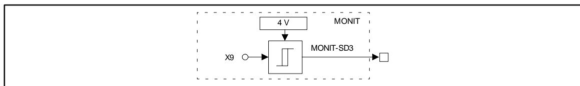
Fig. 7-161 Monitoring of the encoder at X9 (Sd3)
