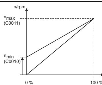
Fig. 5-1 Minimum and maximum speed
