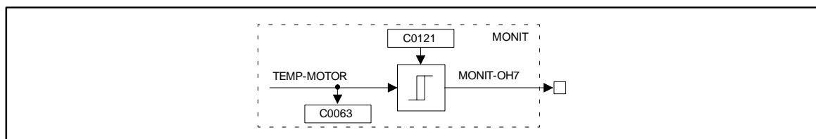
Fig. 7-165 Monitoring of the motor temperature, with adjustable threshold (OH7)
