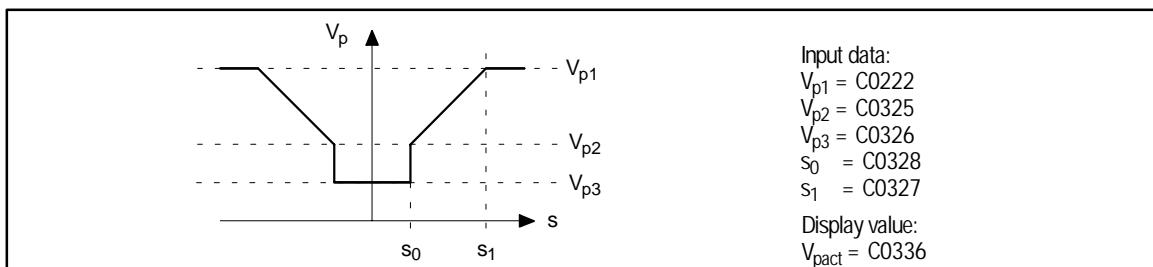
Fig. 7-139 The input of gain  $V_p$  is derived from the process setpoint PCTRL1-SET
