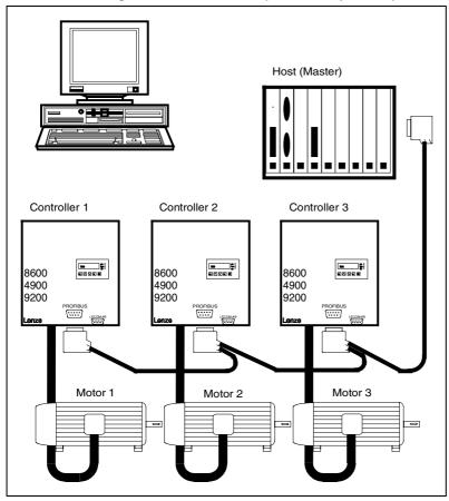
Apart from the RS485 connection you can also use an optical fibre cabling. Here, the Siemens system SINEC-L2FO is used mainly, where point-to-point and star connections (using active star connectors) are possible.
