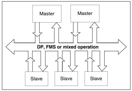
PROFIBUS-FMS is based on the description of objects. Devices are written in as virtual field devices (VFD = virtual field device); with one device having several VFDs. Parameters or variants are displayed as objects, which can be read out or written in using the services "Read" or "Write", when an index (index + subindex) is specified. The FMS device supplies an object description of every variable or data type which contains the most important information about the communication.
