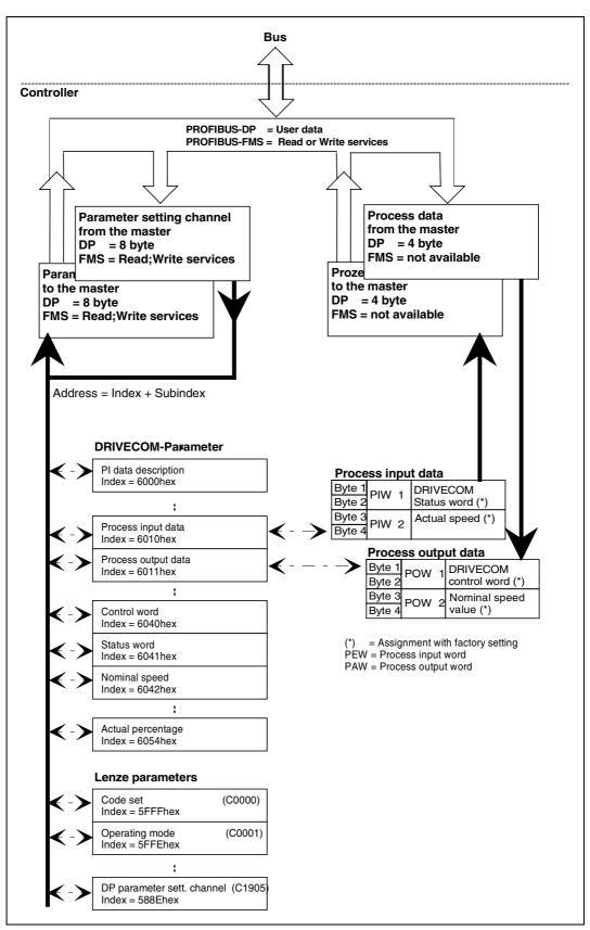
The diagram explains the PROFIBUS access to controller data. Here you have to distinguish between access to process data and parameter data.
