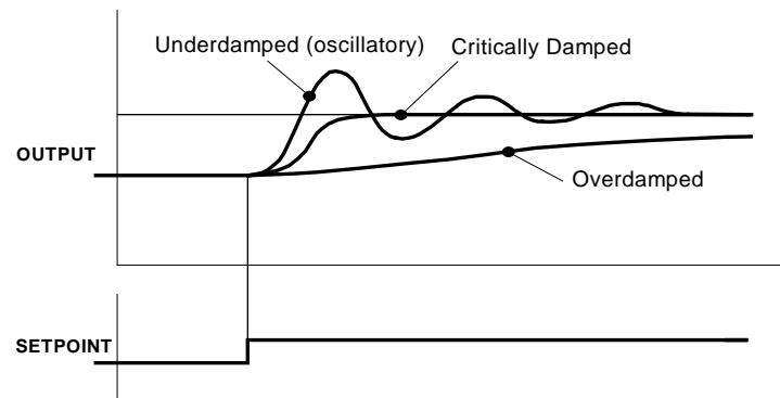
To set up the P gain, set the I gain to zero. Apply a step change in setpoint that is typical for the System, and observe the response. Increase the gain and repeat the test until the system becomes oscillatory. At this point, reduce the P gain until the oscillations disappear. This is the maximum value of P gain achievable.
