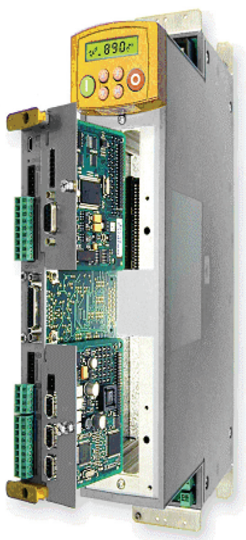
Figure 2. 890 showing Control Board withdrawn, with Options fitted
