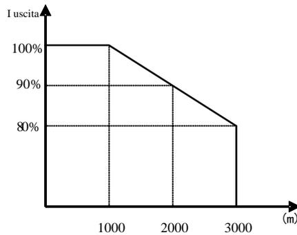
Fig 1-7 Derating Drive's output current with altitude
