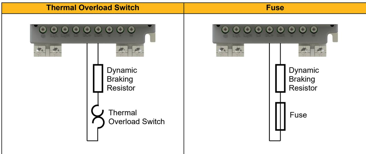
It is recommended the thermal overload switch / fuse is sized with a 10% margin greater than the theoretical continuous current.
