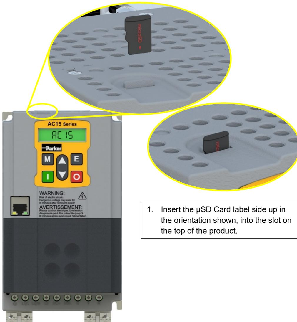
1. Insert the µSD Card label side up in the orientation shown, into the slot on the top of the product.
