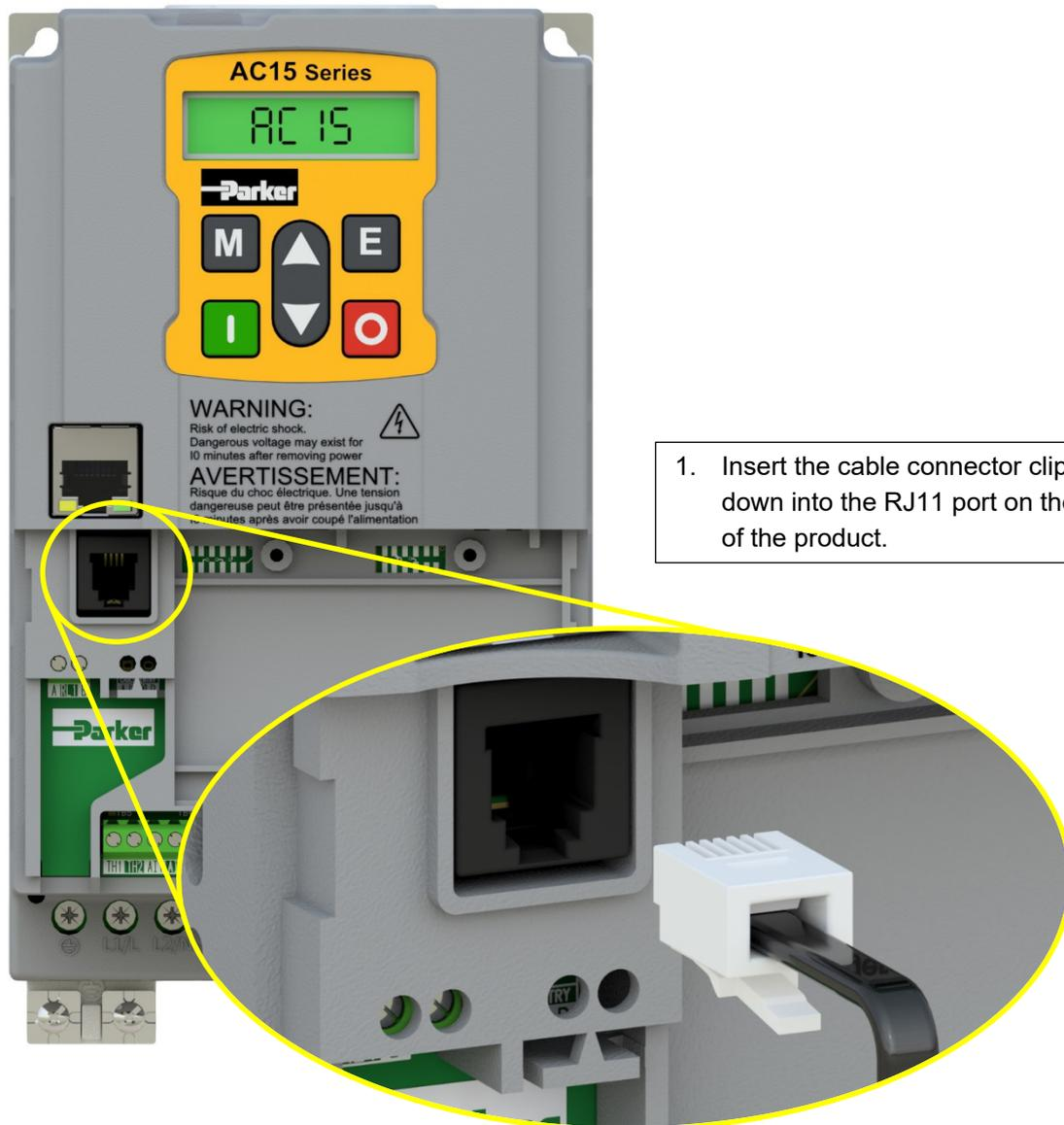
1. Insert the cable connector clip side down into the RJ11 port on the front of the product.
