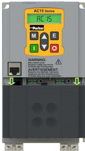
2. Now slide the cover down and pull away from the control module.
