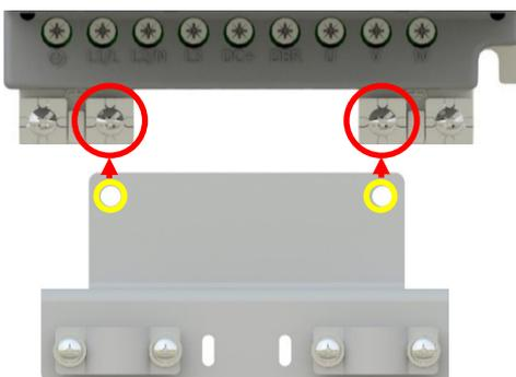
1. Unscrew and remove the necessary chassis PE clamps.
