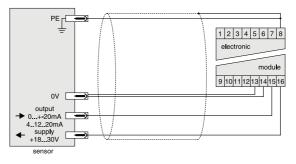
Wiring diagram of sensor input 0...+20 mA / 4...12...20 mA, 2-wire
