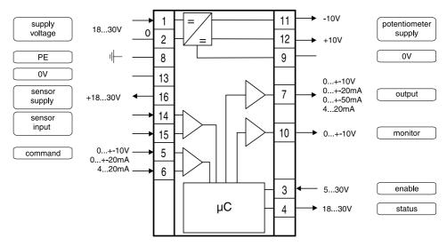
Parker electronic modules PID00A-40\* for rail mounting are compact, easy to install and provide time-saving wiring by disconnectable terminals. The digital design of the circuit results in good accuracy and optimal adaption for closed loop controls by a comfortable interface program. The described electronic unit combines all necessary functions for the optimal operation of closed loop controls.
