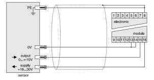
Wiring diagram of sensor input 0...+20 mA / 4...12...20 mA, 3-wire
