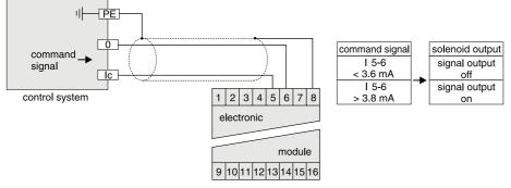
The 4...20 mA option uses the "0 mA" condition as breakdown-information. This means the presence of an evaluable failure information if the input signal line is interrupted. In this case the solenoid output will be switched off. The output will switched on when the input signal reaches a value of 3.8 mA, it switches
