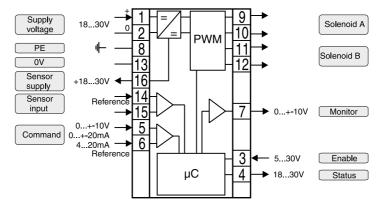
Parker electronic modules PWDXXA-40X for rail mounting are compact, easy to install and provide time-saving wiring by disconnectable terminals. The digital design of the circuit results in good accuracy and optimal adaption for proportional directional control valves with position sensor by a comfortable interface program.
