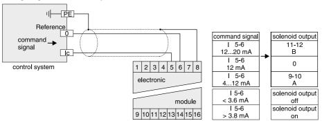
The option 4...20 mA uses the "0mA" condition as breakdown-information. This means the presence of an evaluable failure information if the input signal line is interrupted. In this case the solenoid output will be switched off. The output will switched on when the input signal reaches a value of 3.8 mA, it switches
