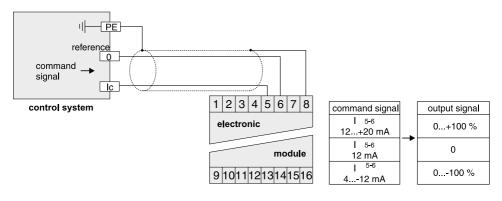
The option 4...20 mA uses the "0 mA" condition as breakdown-information. This means the presence of an evaluable failure information if the input signal line is interrupted. In this case the solenoid output will be switched off. The output will switched on when the input signal reaches a value of 3.8 mA, it switches off when the command falls below 3.6 mA. This
