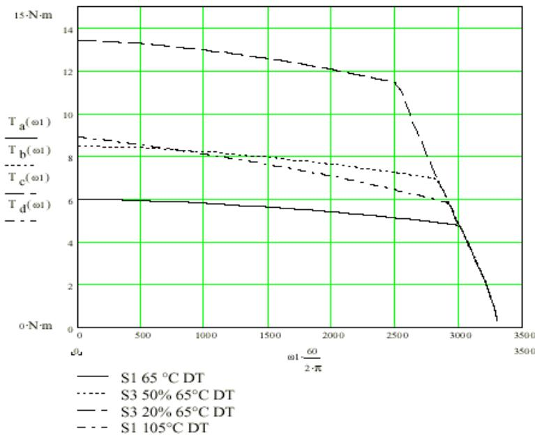
**Characteristic 13****SMH 100 56 06 ...2ID...4: 5600rpm at 400 VAC**
