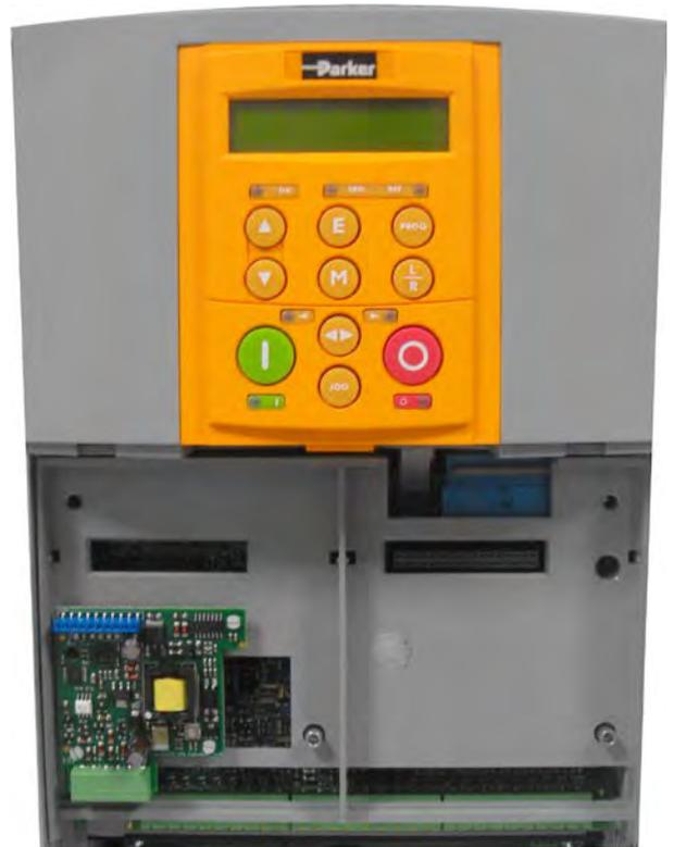
Figure 1 Encoder Receiver Option 590 Mounting
