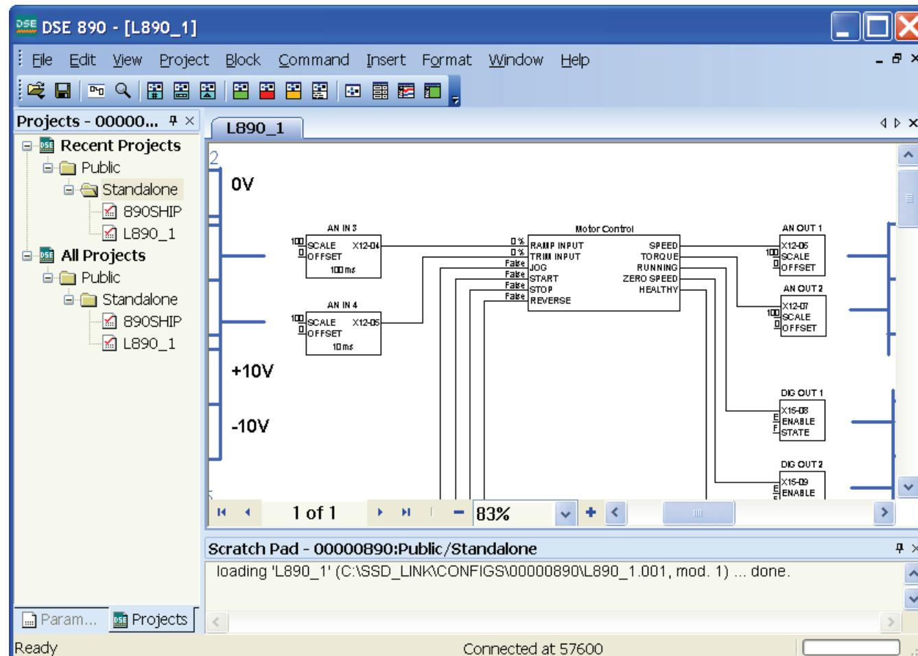
4. Save the configuration by clicking on File/Save or the Save icon, or select "Save" from the "File" menu. This will create a new revision of the configuration, revision 1. The asterisk "\*" against the name will disappear.
