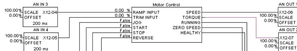
Links are made by connecting an output to an input, in that order.
