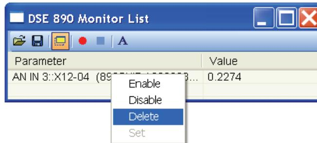
"Set", I available for this parameter, brings up a dialog to change the value. "Enable and Disable allows this parameter to Enabled or Disabled from being updated in the Monitor List.
