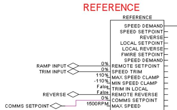
On exiting, the motor Control Macro the additional input parameter "SETPOINT" will automatically appear on the Motor Control block as shown on the right.
