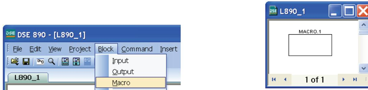
As a result, a new Macro block will be added to your configuration. Double click on the block to open the new, empty diagram. You can add blocks (including further Macro blocks) and links as usual. In addition, you may add input and/or output blocks from the "Blocks" menu using "Input" and "Output" respectively.
