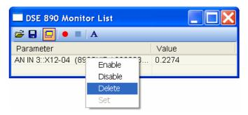
You can easily remove a parameter from the Monitor List by a right click and selecting "Delete".
