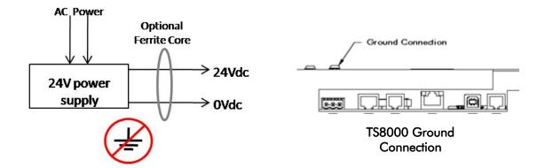
**Important:** Do not connect the power supply common to ground. The TS8000 has its own chassis ground that should be utilized. To further reduce electrical noise, SSD Drives also recommends the use of a ferrite core on the 24Vdc and 0Vdc leads between the power supply and the TS8000.
