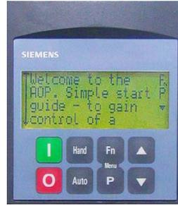
Figure 38. Advanced Operator Panel (AOP).
