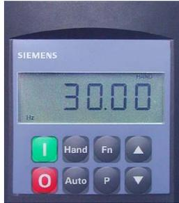
Figure 37. Basic Operator Panel (BOP).
