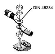
Image 6-2 Connection of auxiliary terminals with cable lug
