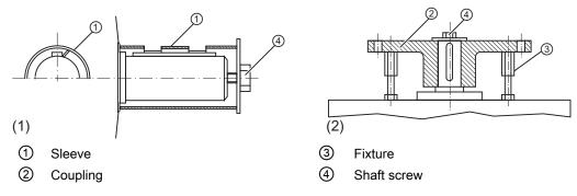
Image 4-1 Rotor shipping brace without coupling (1) and with coupling (2).
