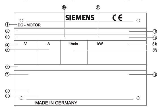
Image 3-2 Schematic rating plate
