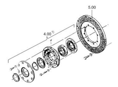
Image 10-3 Rolling-contact bearing for 1G.5, 1H.5, shaft heights 500 to 630
