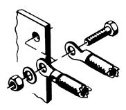
Image 6-1 Connection of main terminals with cable lug
