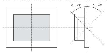
For inclined installation in horizontal format, the following ambient temperatures are permitted:
