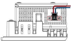
Secure the connection terminal with the marked screws.
