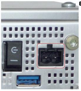
Connect the connection terminal at the marked position.
