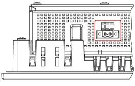
Connect the connection terminal at the marked position.
