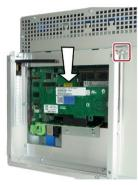
5. Push the PCle card holder in the direction of the PCle card and secure this with the marked screw.
