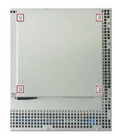
2. Remove the marked screws and pull out the blanking plate.
