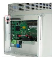
4. Insert the PCIe card in the direction of the arrow and secure this with the marked screw.
