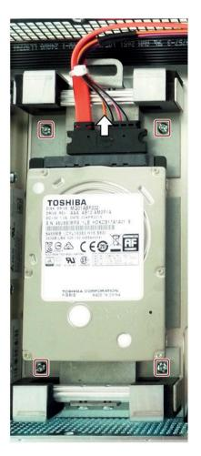
4. Detach the hard disk from the base plate. Remove the four screws that connect the hard disk and the base plate.
