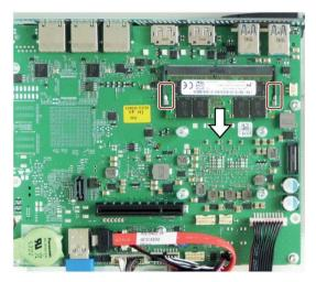
6.2 Installing and removing a memory module
