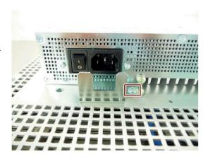
3. Insert the power cable into the socket and fasten the power plug fastener with the marked screw.
