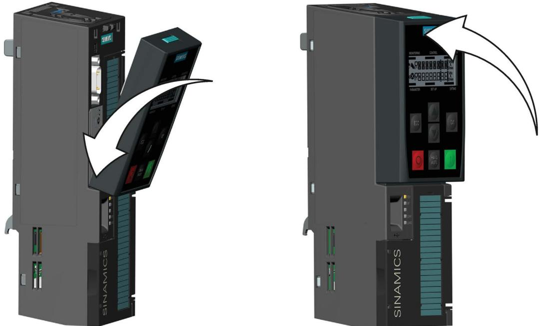
Image 5-1 Fitting the BOP-2 to the Control Unit
