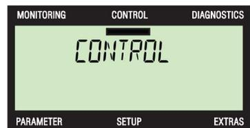
The Inverter must be in HAND mode before any functions can be accessed. If HAND mode is not selected a notice screen is displayed stating that the Inverter is not in HAND mode.
