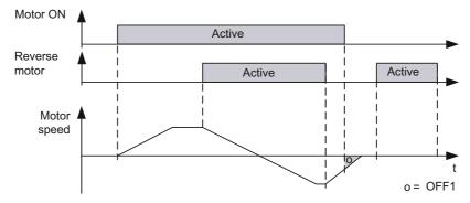
Figure 5-2 Two-wire control using digital inputs, method 1
