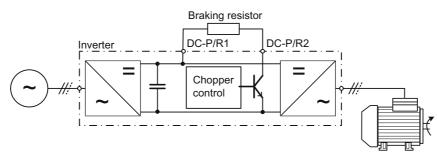
Figure 5-11 Dynamic braking with braking chopper in the inverter
