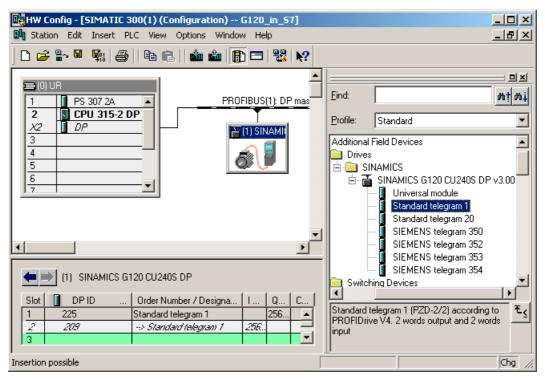
Add the required telegram type to slot 1 of the inverter by dragging and dropping it from the HW catalog.
