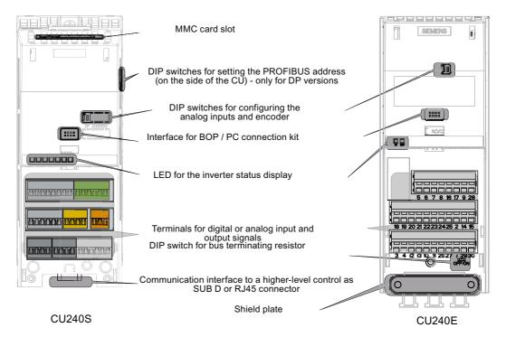
Figure 3-3 User interfaces of the CU240E/S
