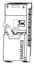
3.4 Installing the Control Unit
