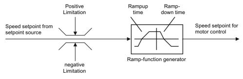
Figure 5-8 Setpoint calculation in the inverter
