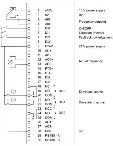
Figure 4-1 CU240E terminal overview: wiring example for using the factory settings
