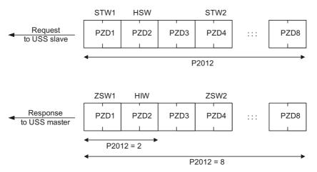
Figure 5-20 USS process data channel
