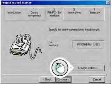
Figure 4-5 Setting the PC interface
