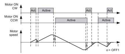
Figure 5-4 Two-wire control using digital inputs, method 3
