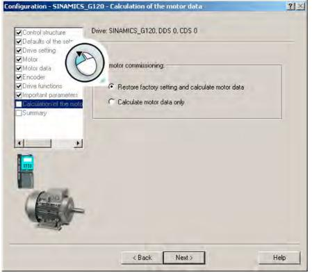
Figure 4-14 Calculating the motor data and restoring the factory setting
