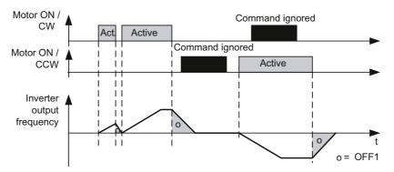
Figure 5-3 Two-wire control using digital inputs, method 2
