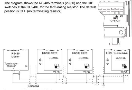
Figure 5-17 USS network via RS 485
