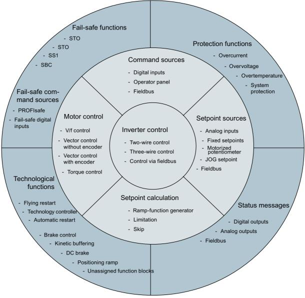
Figure 5-1 Overview of inverter functions
