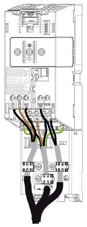
Figure 3-2 Shield connection kit FSA
