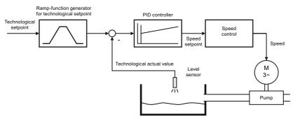
Figure 5-14 Example: technology controller as a level controller
