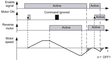
Figure 5-6 Three-wire control using digital inputs, method 2
