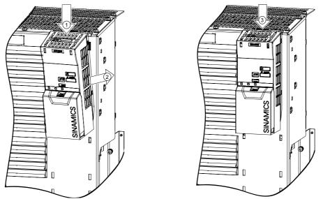
The Control Unit is simply snapped-on to a Power Module. This also establishes all of the electrical connections between the two components.
