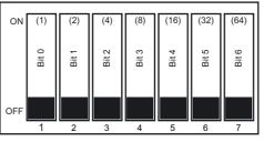
Figure 5-21 PROFIBUS DIP switches
