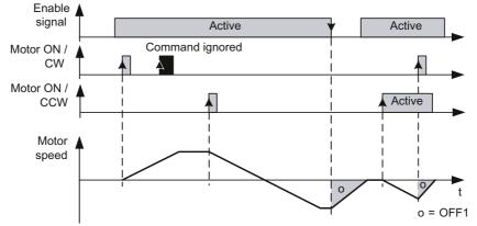
Figure 5-5 Three-wire control using digital inputs, method 1
