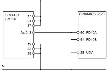
Figure 5-46 Connecting up an F digital output module in a control cabinet
