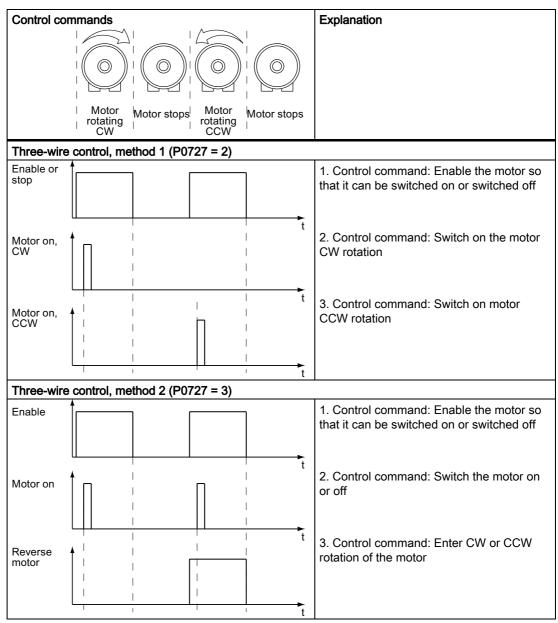
Table 5-2 Comparison of the methods for three-wire motor control
