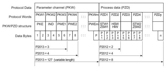
Figure 5-19 USS user data structure
