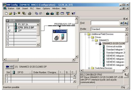
Figure 5-29 Connect G120 to the PROFIBUS network
