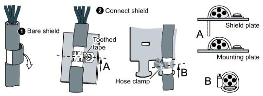
Figure 4-2 Examples for EMC compliant shield support
