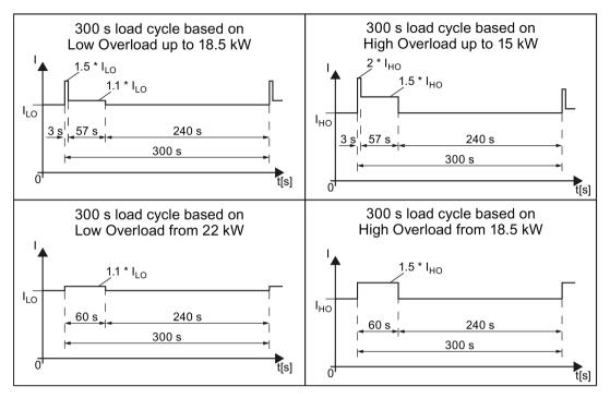
Figure 7-1 Duty cycles, "High Overload" and "Low Overload"
