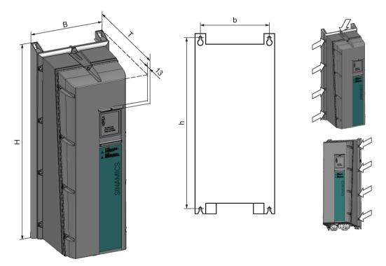
Figure 4-3 Dimension drawing FSA ... FSC
