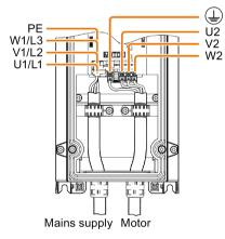
Figure 5-5 Connections for PM230 Power Modules, FSA ... FSC
