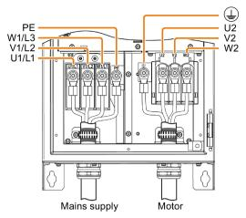
Figure 5-7 Connections for PM230 Power Modules, FSD ... FSF
