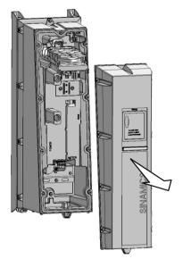
2. Remove the cable gland plate from the bottom of the inverter.
