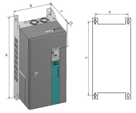
Figure 4-4 Dimension drawing FSD ... FSF
