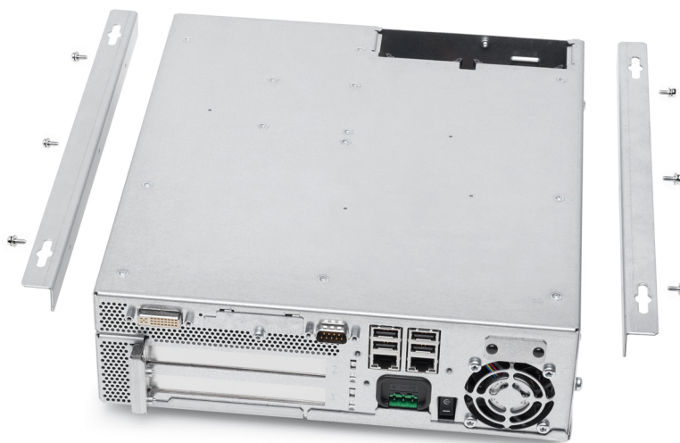
Figure 14-13 PCU 50.5 with bracket for flat mounting
