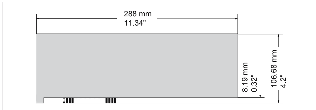
Figure 13-40 Maximum size of PCI module (only possible on slot 1)
